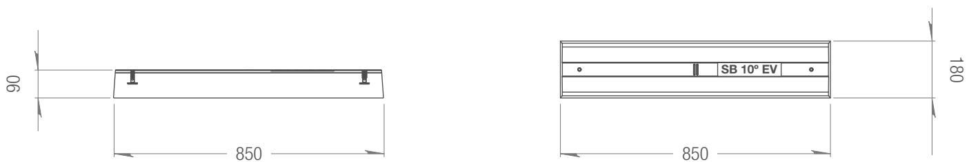
**ABMESSUNGEN DES BALLASTS 23010.EP**
