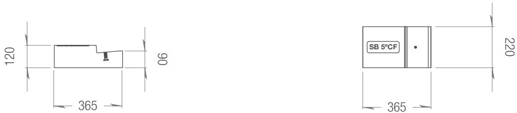
**ABMESSUNGEN DES BALLASTS 23005.CR**
