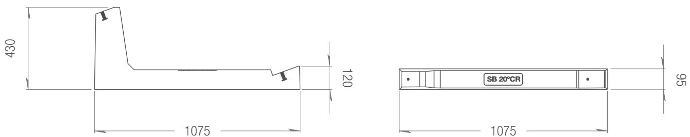
**ABMESSUNGEN DES BALLASTS 23020.CRT**
